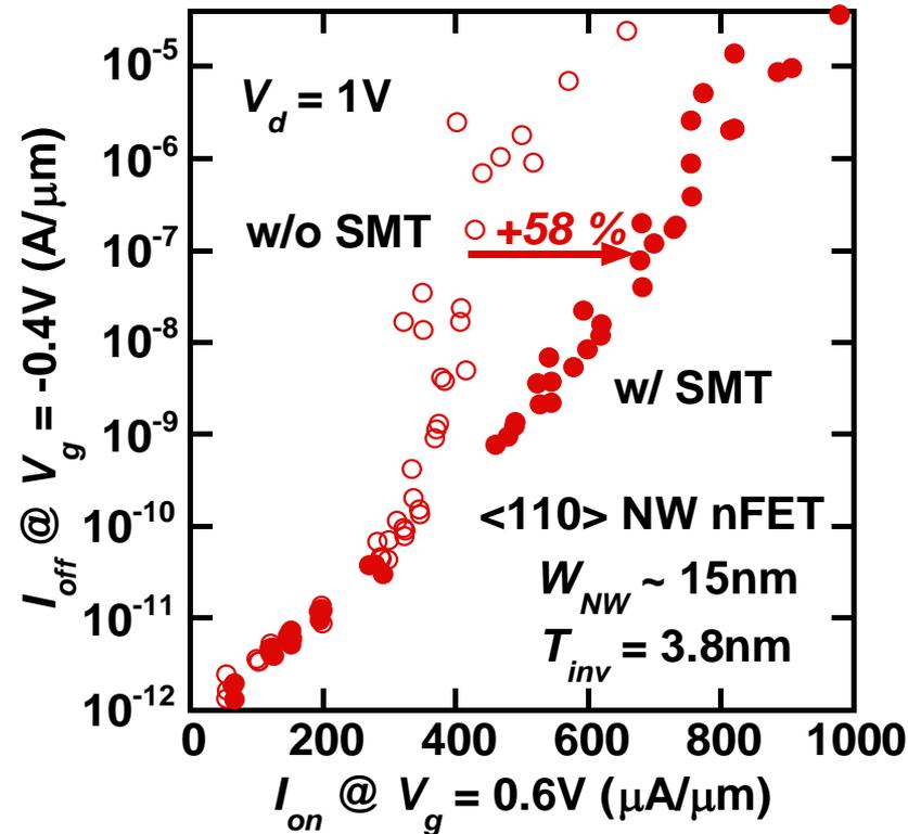
Stress engineering to nanowire channel is highly effective for the performance improvement of nanowire transistors.
