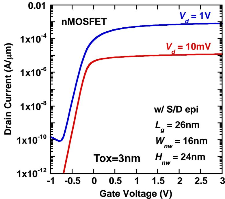
Wire width reduction leads to steeper subthreshold swing
