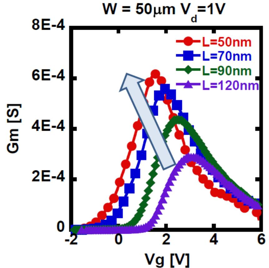
Gmmax increased by a factor of 2 by Lg scaling
