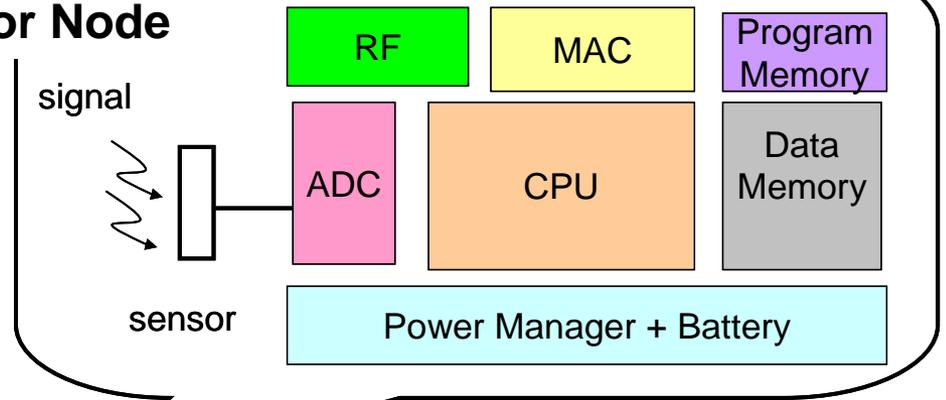
Vast numbers of sensors, active for several years with a tiny battery or a solar cell (ex. 10mW level, 100kbps 10m Wireless Network)
