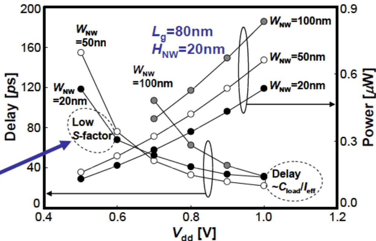
In the low  $V_{dd}$  operation, the sub-threshold characteristic is a key in the circuit performance.
